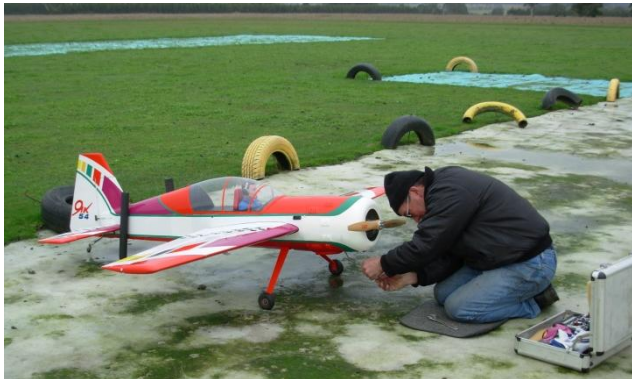
I think Max is doing a plug change on the 3MM 53cc engine after having some trouble getting it to run reliably.
