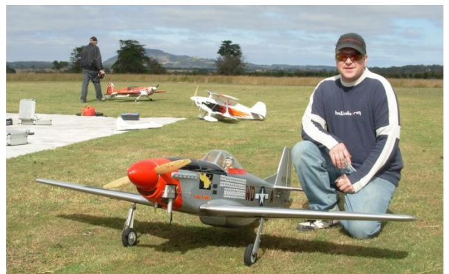
Mat Werner with his new 80.5" DLE30 powered P51 with flaps and retracts.
