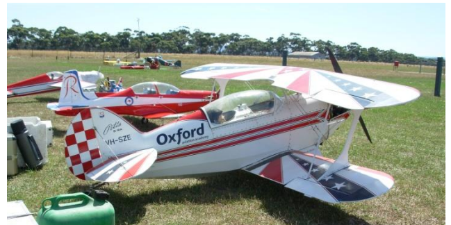
David Law’s ¼ scale Pitts S2A, powered by a 100cc twin. Model is entered in this year’s world scale champs to be held in Spain during August.
