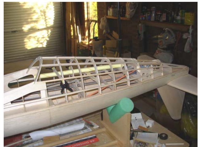
Photo taken prior to sheeting the lower fuselage. I didn’t think the kit had enough frames so intermediate frames were fabricated and fitted.
