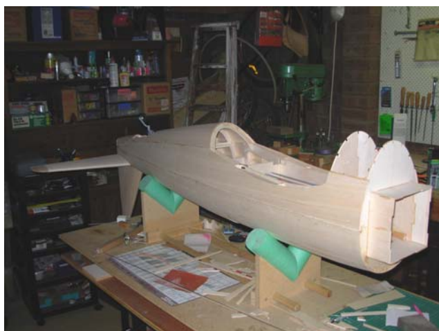
Firewall is now ready to be fitted and allowance has been made for cockpit detail.
