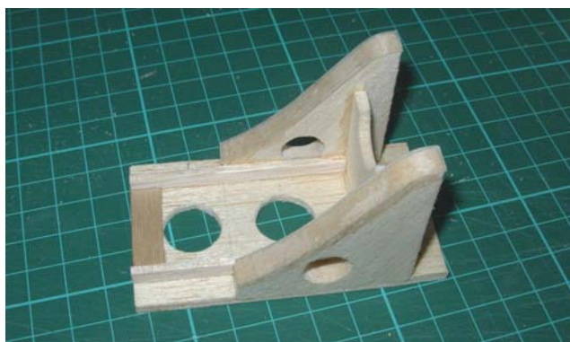
Tail wheel retract guide assembly to centralize tail wheel as it retracts. The tiller arm contacts the ramps holding the wheel in the centre. Required because steering cables slacken as it retracts allowing wheel to rotate and foul on airframe structure.
