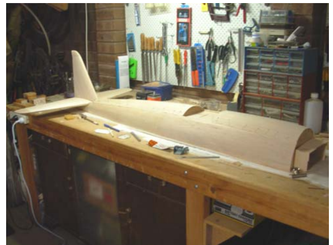
Upper fuselage is built on the work bench – tail plane and fin are also fitted while on the bench.
