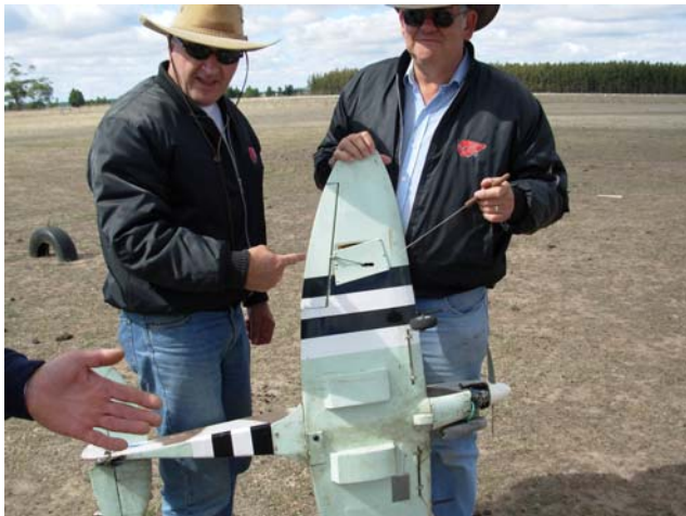
How lucky is that! Aileron servo plate came adrift in flight.
