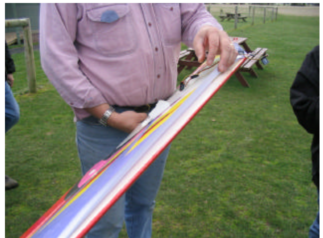
You might not be able to see it, but Rick's index finger is holding back the offending loose covering that caused the Swallow to crash. Fortunately model is quite repairable.
