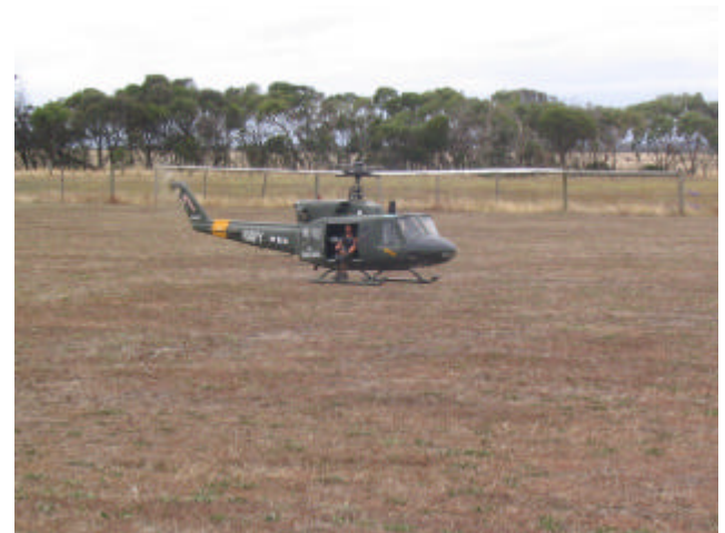
Mario’s Iroquois powered by a Zenoah 23cc – weighs 9.5 kg
