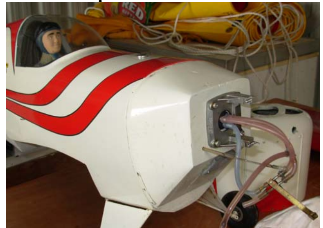
The engine mounting beams have broken through the attachment holes. Loss of strength must be a consideration when filing engine beams to provide crankcase clearance.
