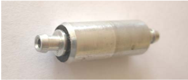
Fuel filter was drawing air through the seal.
