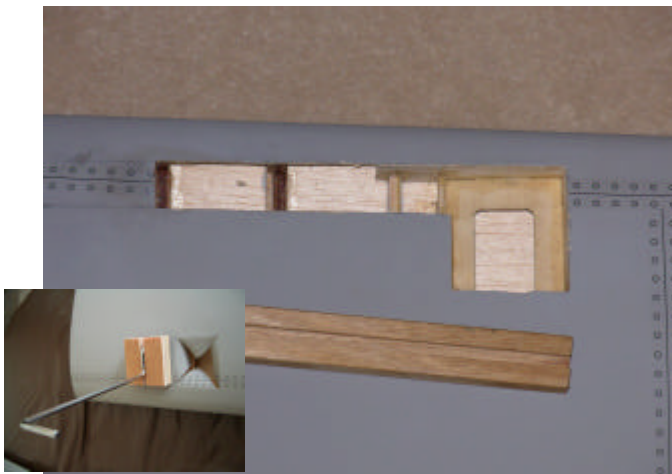
The photo inset, shows how the landing gear was designed to be fitted and was clearly unsatisfactory. The redesigned landing gear shown will use a more conventional landing gear block and long torsion bar.
