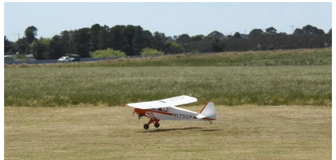
And touch down – note the up elevator.
