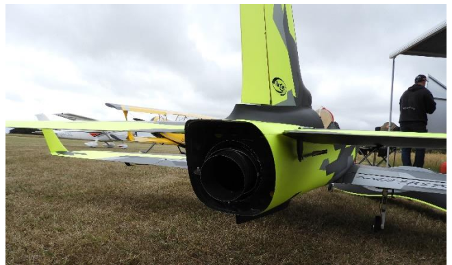
The Mephisto has a vectored thrust nozzle which enables 3D type manoeuvres. I think Steve said he wasn't using it just yet.
