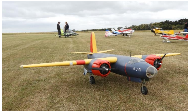
The B-26 is powered by two Saito 115 four stroke engines.
