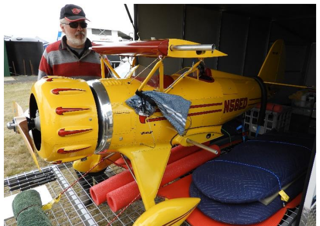
Peter Evans drooling as I was at the 1/3 scale WACO YMF-5 powered by a Moki 250cc radial engine.
