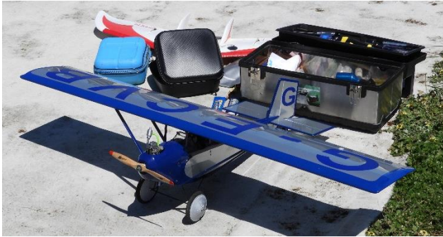
Nigel's Pietenpol Aircamper supplied by Hobbyking on Sunday 11 th November. Model has a wingspan of 1370mm and is powered by an OS26FS.
