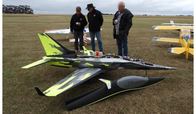
Max, Graeme & Ted looking over the inner workings of Steve Wilcox's CARF Models Mephisto Jet. It's powered by a KingTech K-310 turbine having a maximum thrust of 31 kg.
