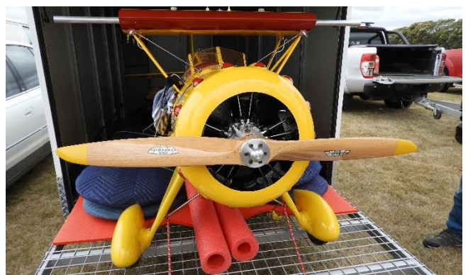
Undercarriage consisted of working oleos within each leg as per the full size.
