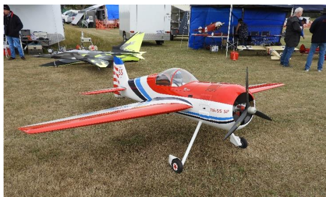
Large (around 3m) Yak 55SP aerobatic ship – DA twin cylinder engine.
