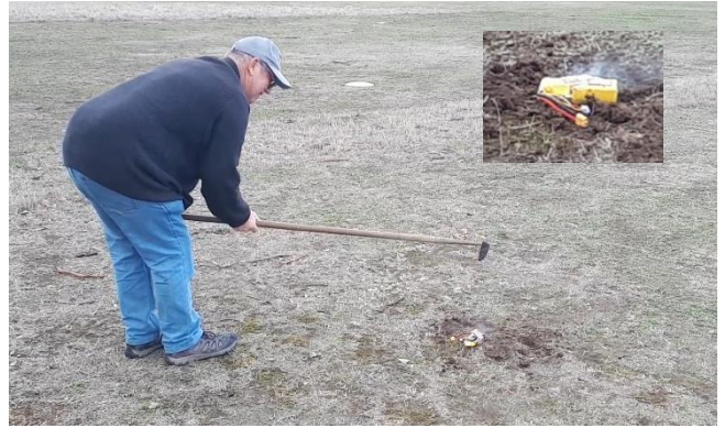
Peter Weston trying to smash the cells with a mattock to short them out.
