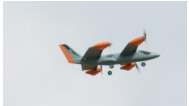
The V-Hawk X4 has transitioned to fixed wing mode and is now flying like a convention aircraft.
