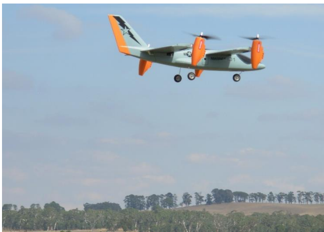
After climbing to 30 or 40 feet it is about to transition to fixed wing flight mode.
