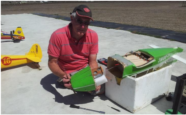
Fortunately the wood around the break wasn't fuel soaked which would have made a strong repair hard to achieve. (BTW. Auto degreaser does a pretty good job pulling the oil out of oil soaked wood, also good for cleaning fibreglass cowls etc. prior to repairs.)
