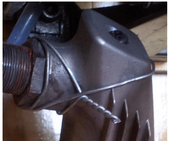
Close up of lock wire around lock nut and muffler of OS 155 Alpha. Hopefully it is successful in the long term.
