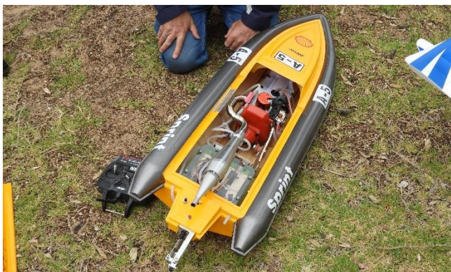
A close up shot the engine and radio installation. The radio gear is housed in a watertight compartment at the stern.
