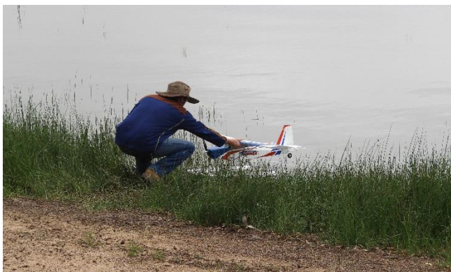
Alan was the first to fly. His model had reverse thrust so it could push itself out and turn around for take-off.
