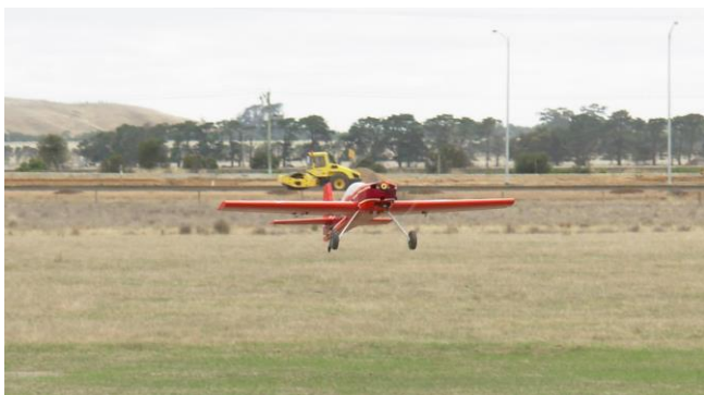
The Extra coming in to land under extreme difficulty being so tail heavy and not enough down trim available. It turned out to be a very nice landing although this was at least the third approach.
