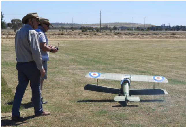
Graeme taxiing out Jeff's Sopwith Camel. Seemed to taxi okay but as soon as the power was applied and started to roll faster it nosed over.
