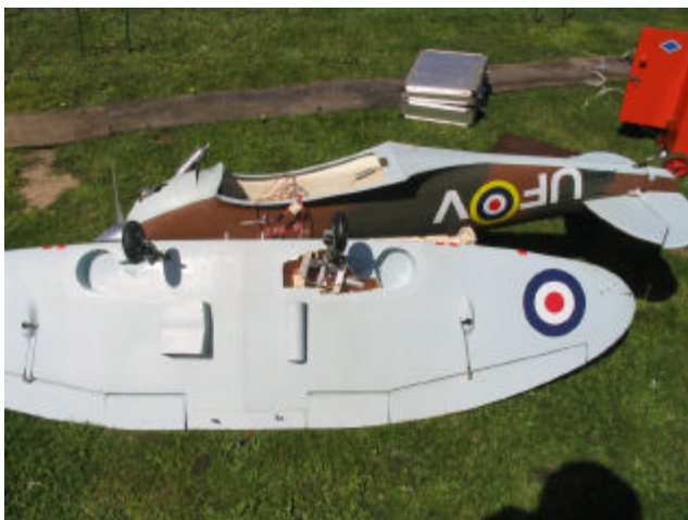
Glenn's Spitfire after wing was removed. The only damage sustained was to starboard landing gear mounting.
