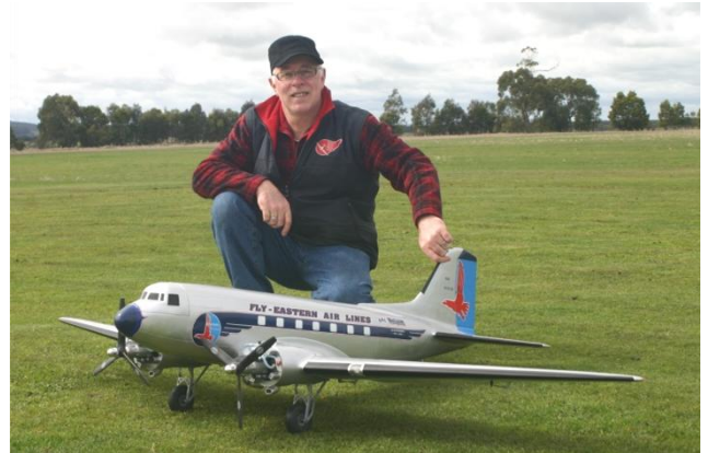
Wayne Goodwin with the DC3 he has built from the Top Flite Gold Edition kit. Model has a wingspan of 82.5", is powered by two Magnum 52 four strokes and is fitted with Robart retracts especially designed for the DC3.
