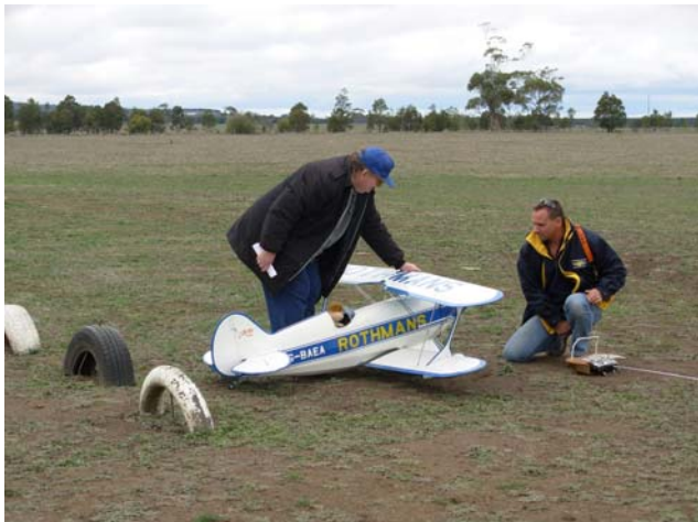
David Law is starting the 3W 100cc twin cylinder petrol engine in his impressive Pitts Special with Noel Whitehead holding on. Model must be about 1/3 scale.
