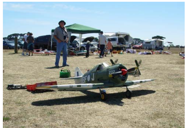
John Hoy's (Warrnambool Club) big CAC Boomerang powered by a Zenoah 62 petrol engine. Model flew impressively on Saturday but engine mount problems prevented further flights on Sunday. John finds it a challenging model during takeoff and landing.
