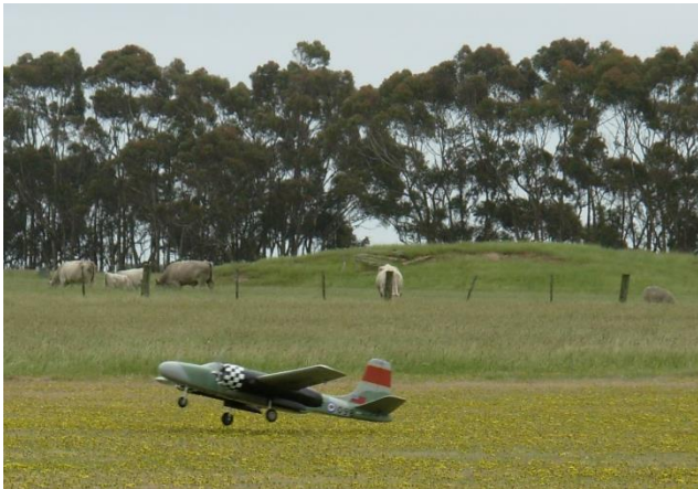
This might be the last photo ever taken of this model (B25 Mitchell) in one piece. I just managed to snap it as it lifted off before climbing fairly steeply, rolling over and going in vertically from about 40 feet. This happened just before the presentations and totally unexpected, I thought to myself could it be reversed ailerons and apparently it was the wrong model selected in the transmitter, so effectively reversed ailerons.
