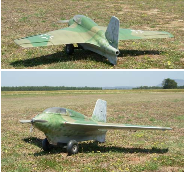
Two more shots of the Komet, the lower one shows the dolly that drops away on lift off.
