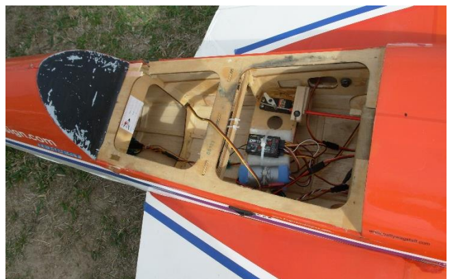
Front aluminium locating pin vibrated out allowing the canopy to lift up at the front tearing out the rear attachments.
