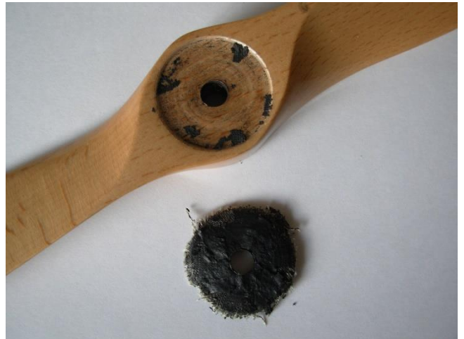
The rubber washer was gradually disintegrating as it slipped.
