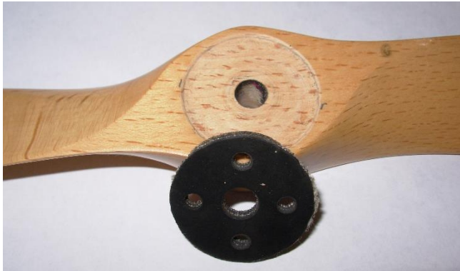
Reinforced rubber washer to try and stop prop driver digging into wooden propeller hub.
