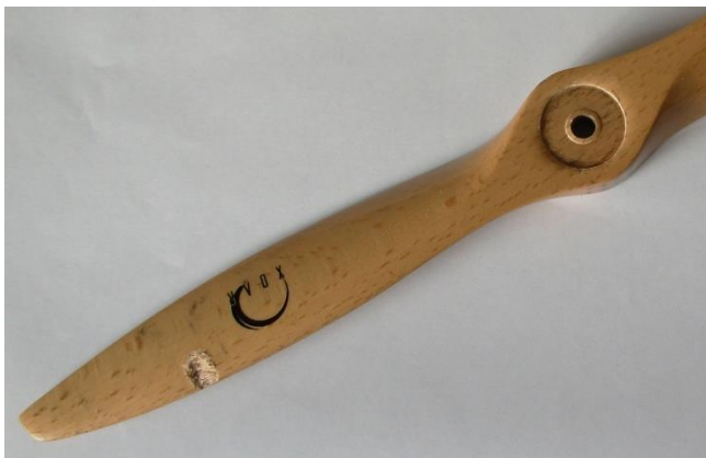
The locknut flung off and damaged the blade – actually cracked on the other side. The retaining nut washer has also left a deep imprint in the hub. If the washer was a little larger in diameter it would help.
