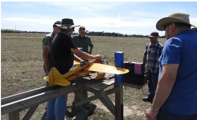
Wayne had a go trying to tune the OS46AX but it was an uphill battle with air bubbles entering the fuel line between needle valve and carburetor.
