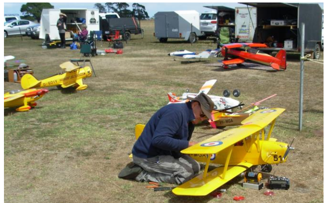
Murri had to do a little bit of work on the Tiger Moth rigging after a forced landing when the engine quit. It seems the 91 four stroke has a tendency to overheat when the cowl is fitted. The owner of the red Pitts in the background (from Melton I think) put on a superb aerobatics display and flew the jet to the left as well.
