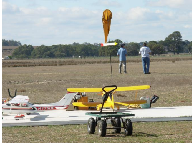
Note the coloured arrow attached to the wind sock pole that can be turned to indicate the duty runway.
