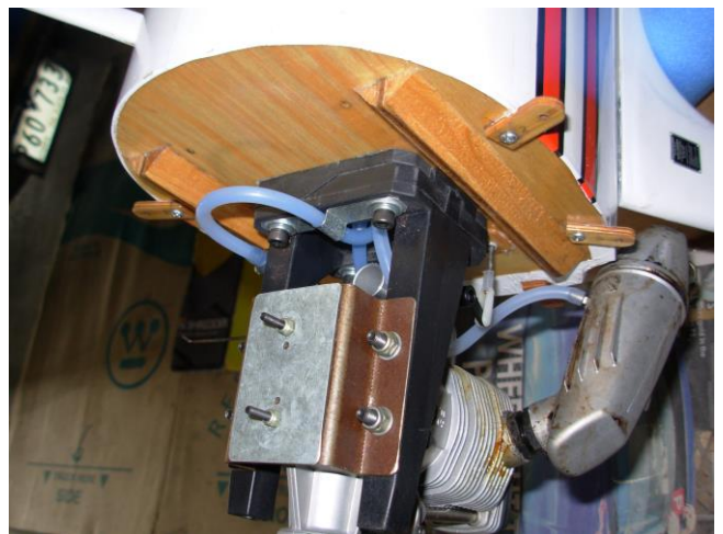
Same thing was necessary on my Great Planes Super Stearman. On this model, GP suggest and in fact provide a plywood box to mount on the firewall above the engine mount to hold the 18oz lead they found necessary. What crap is that!!! With the OS200 it didn't need much anyway.
