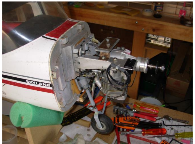
Use a steel 'hat' section to clamp any lead that is needed for ballast. That's what I did on my Top Flyte Cessna 182.
