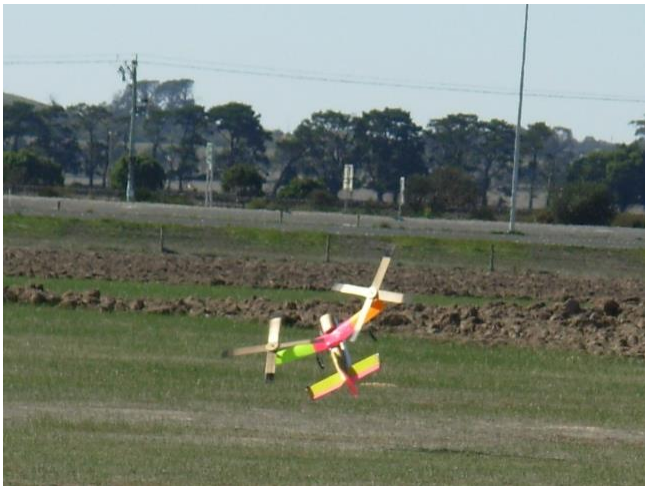
It was all over pretty quickly. Too much lift on the right wing rotor or maybe not enough on the left. It did leave the ground briefly though before going in on the left rotor – don't think it did any damage.
