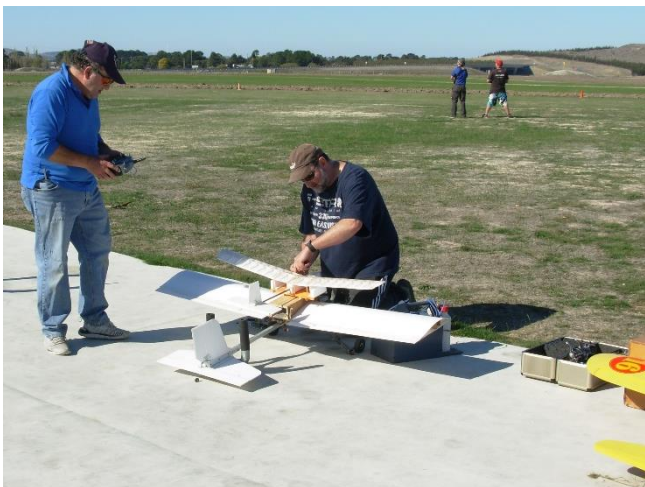
Greg Savige had his core flute constructed powered model and glider attached on top with release mechanism at the field for another try out. Nick volunteered to fly the glider once released.
