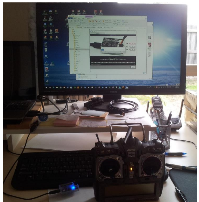
Once the transmitter was plugged in when the HPP-22 program requested it, it all started to happen. The LED on both HPP-22 module and transmitter switch flashed rapidly until the whole process finished.
