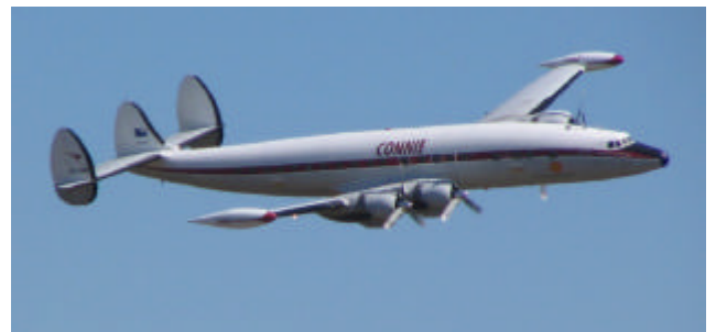
This is a site that will bring back memories for many. The Super Constellation had 3 fins so the height could be kept low to enable the aircraft to fit into existing hangars.
