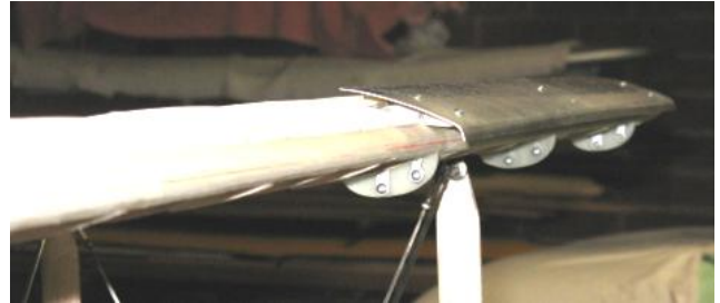
The leading edge slats are designed to pop out when the angle of attack reaches a critical value. This maintains a more laminar flow over the wing upper surface to mitigate tip stall.
