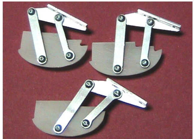
Slat mount control arm assemblies – 3 per slat. The geometry is critical to get the desired motion.
