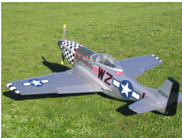
Graeme's (aka Al, no Al aka Graeme) giant scale Top Flite P51 powered by US 41cc petrol engine shortly before maiden flight. These are quite an impressive kit.
