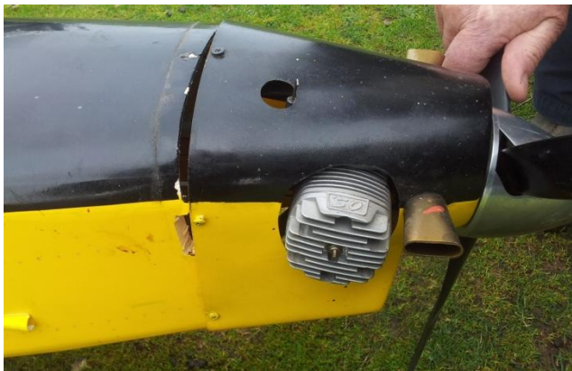
The firewall pulled away from the fuselage structure mid flight causing drastic trim change. Model is a VQ Pilatus Porter powered by an OS 160 FX.
