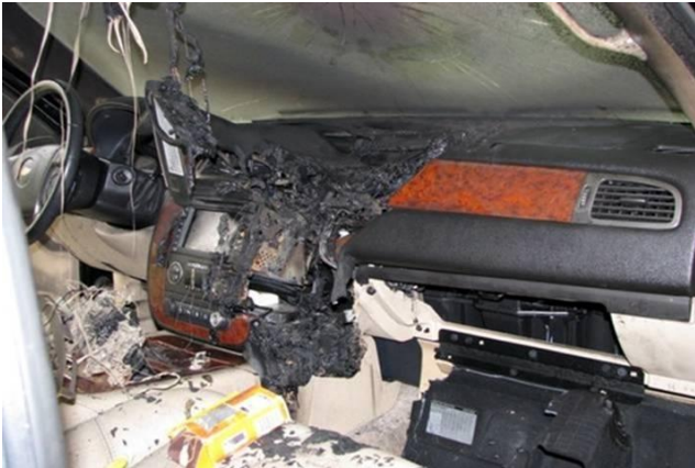
This is what happened to a car after the battery in the GPS ignited after being left in the hot sun. Scary stuff. I guess similar to the battery fires in the 787 Dreamliner.
