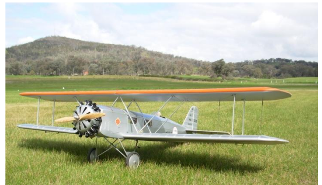
This is David Balfour's latest scale model. A Boeing 40C powered by an OS200FS. With the recent inclement weather David hasn't been able to test fly it but no doubt that will change very soon. The first Model 40 was built for a 1925 U.S. Post Office competition as a replacement for the converted military de Havillands that had carried the airmail since 1918.
