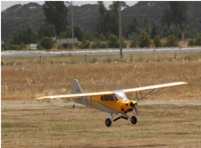
Graeme's new Hangar 9 Carbon Cub at the field on Sunday 7 th January. Powered by an ASP91 four stroke.
