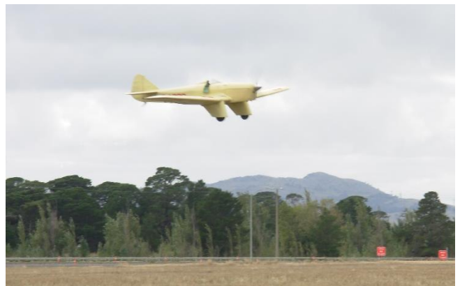
Glenn's now veteran Miles Hawk on a fly pass over the strip. It's now powered by a DLE35 instead of the original Zenoah 22cc.
