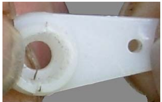
You can see the crack through the spline, which we have deduced was there prior to the crash due to the dirt inside.
